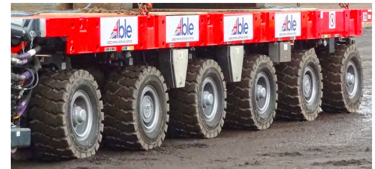
ABLE's 6 Line Scheuerle SPMT
